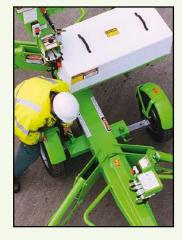
Retractable axles allow the **120** to pass through a 1.10m (3ft 6in) wide opening.
